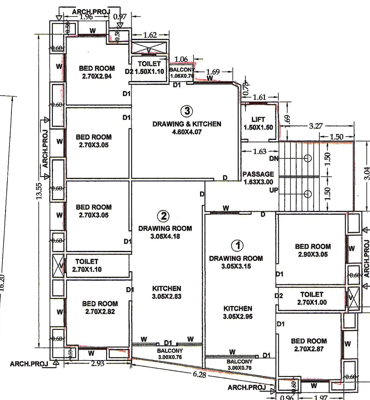
TYPICAL FLOOR PLAN (FIRST FL. TO FIFTH FL.) F.S.I. AREA: 131.25 SQ.MT. BUILT UP AREA: 150.88 SQ.MT.
