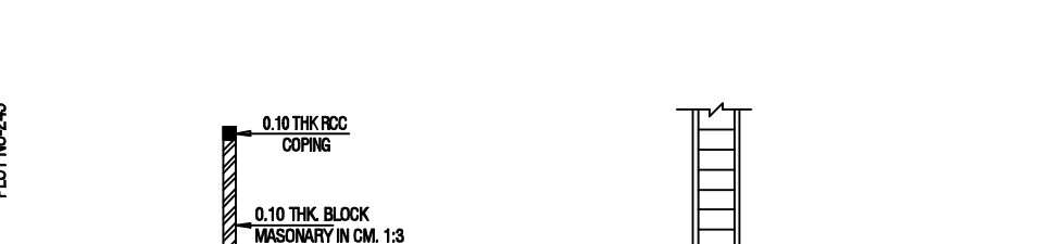
FOUNDATION DETAIL FOR COMPOUND WALL SCALE 1:50
