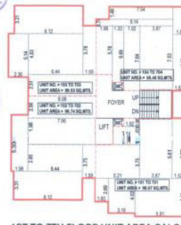
1ST TO 7TH FLOOR UNIT AREA CALC
