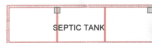
- SEPTIC TANK (50'0" X 12'0" X 5'0" Depth)
