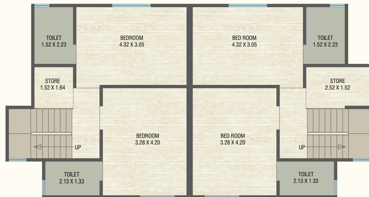
A-TYPE FIRST FLOOR PLAN B.U.A. - 48.46 SQ.MT PLOT NO. 1 TO 5,8,9,12,13,16,17,18,19,20 = 14 UNITS
