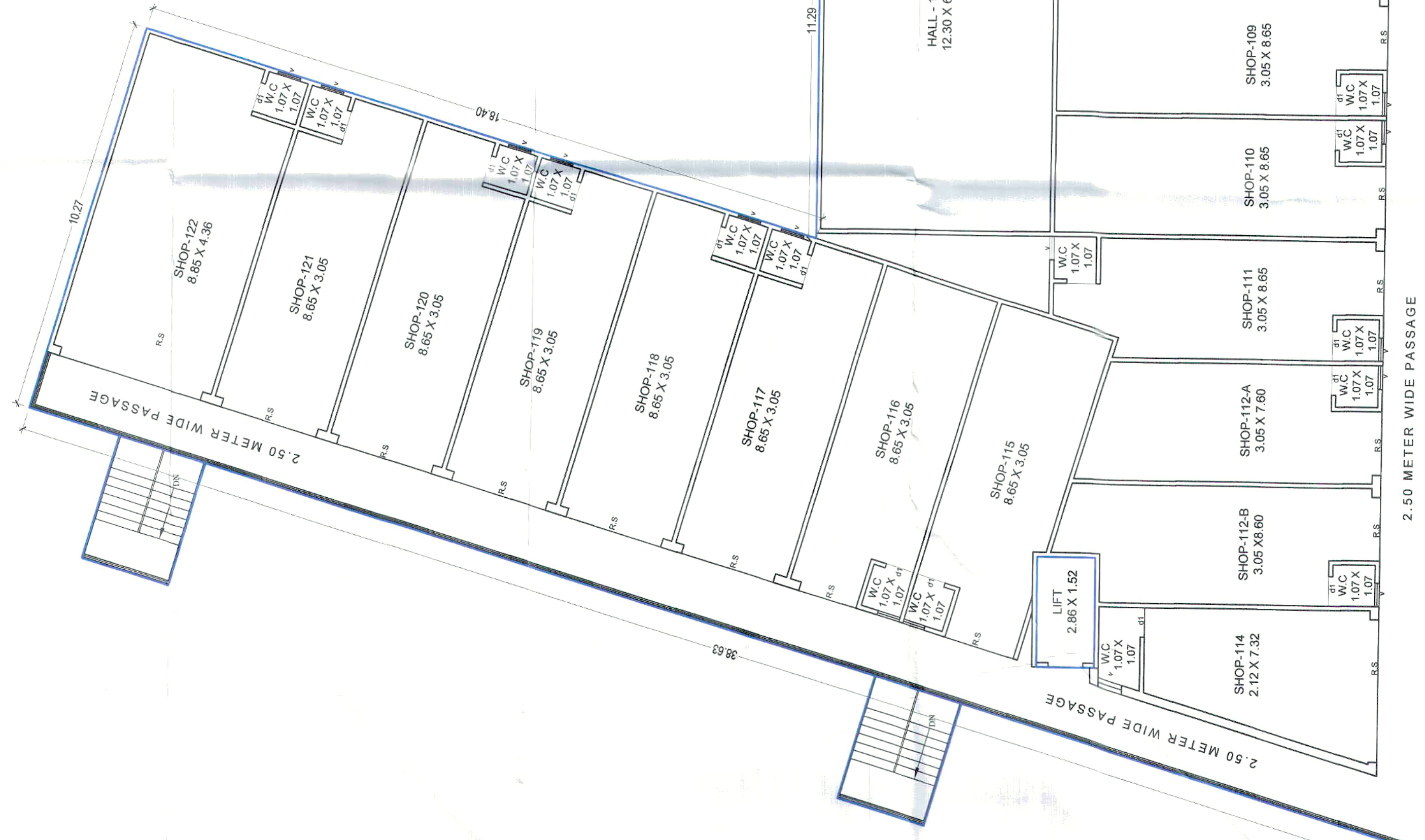
EXISTING 1st FLOOR PLAN B.U.P AREA [942.05+27.61] = 969.66 sq.mt. F.S.I AREA = 942.05 [comm.] TOTAL F.S.I AREA = 942.05 sq.mt.
