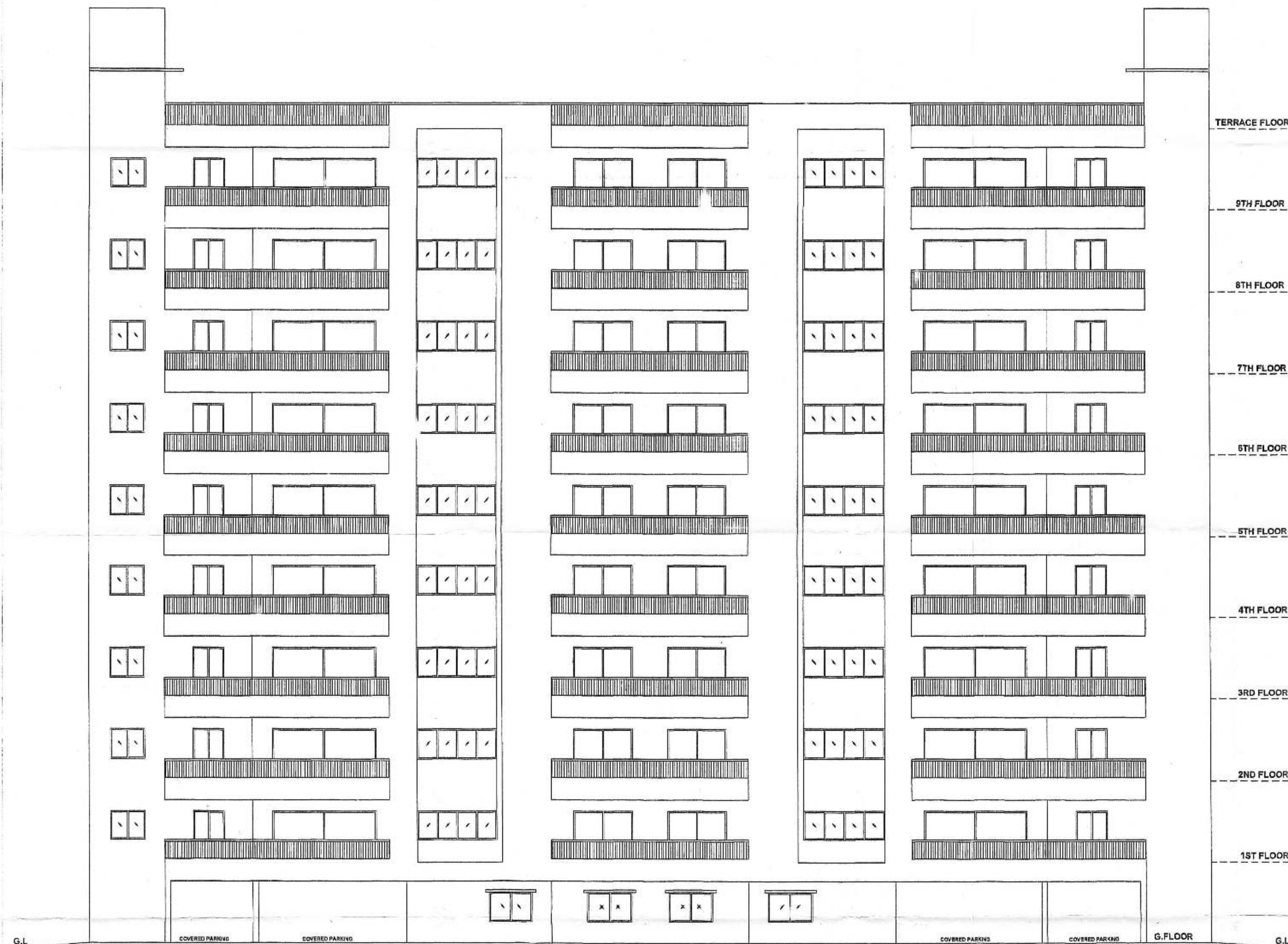
FRONT ELEVATION SCALE= 1:100 (BLDG.B)
