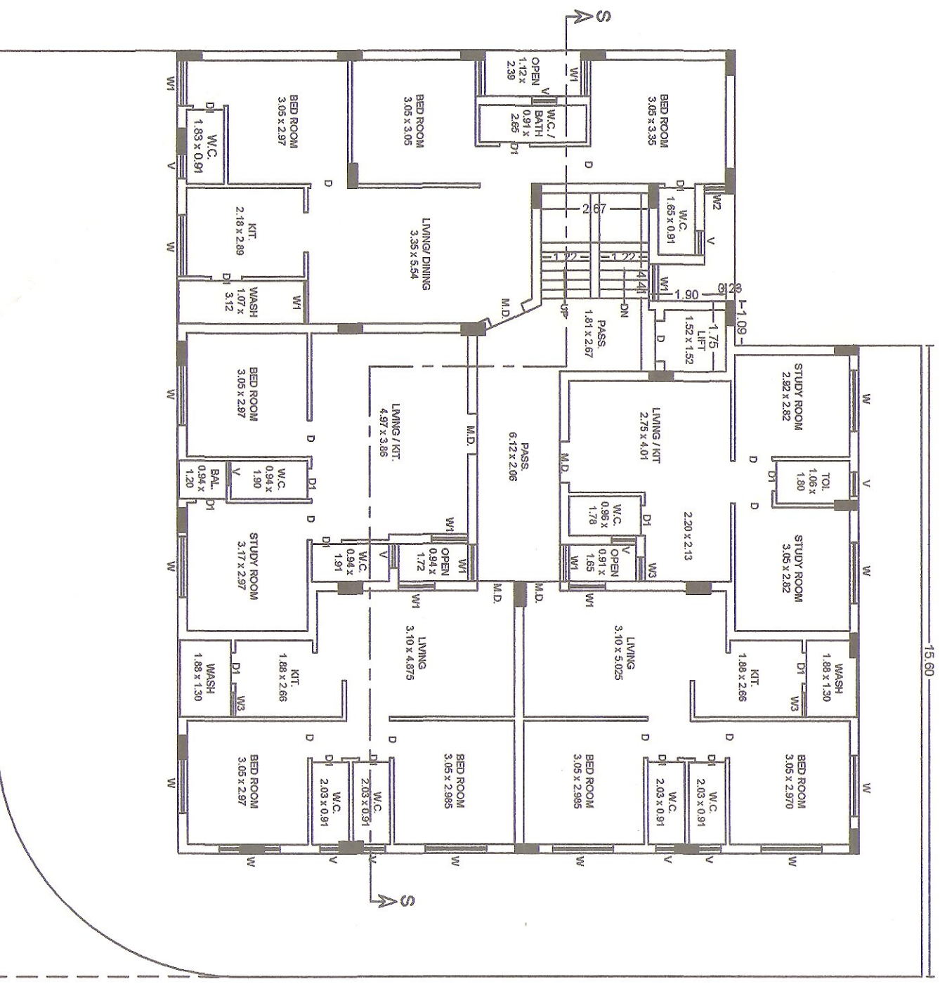
1st to 3rd Floor Plan SCALE 1:100
