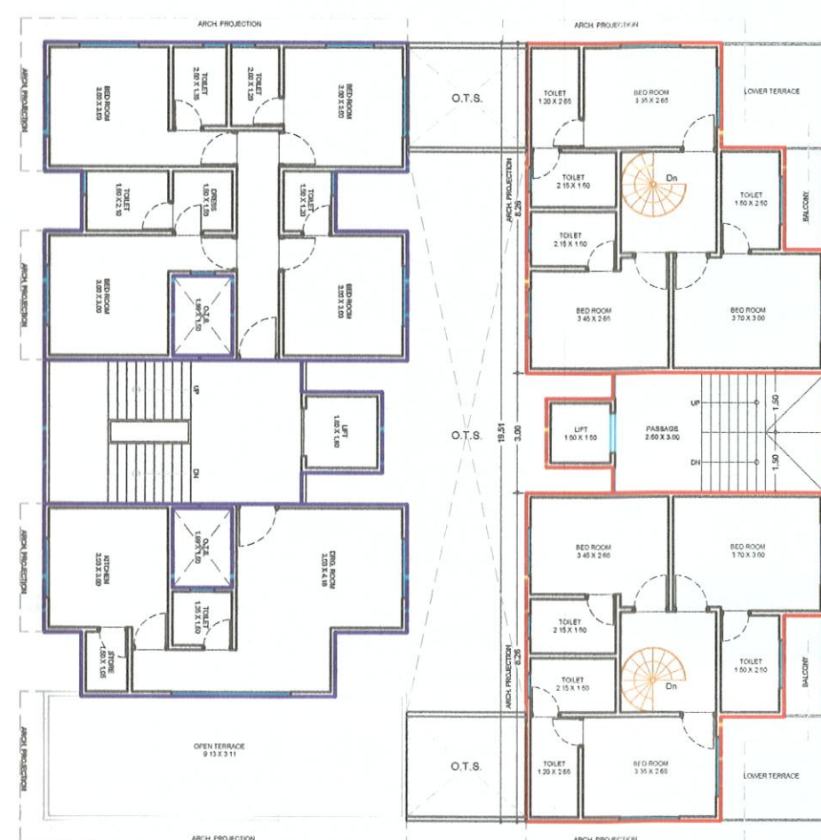
PROP. EXTN. 7TH FLOOR PLAN BUILT UP AREA : 123.78 SQ.MT F.S.I. AREA : 104.90 SQ.MT.
