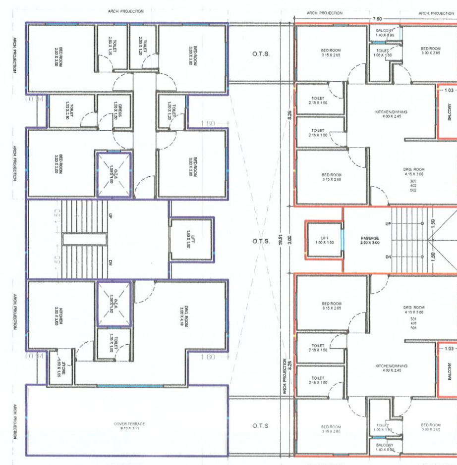
PROP. EXTN. 5TH FLOOR PLAN BUILT UP AREA : 137.72 SQ.MT F.S.I. AREA : 116.84 SQ.MT.
