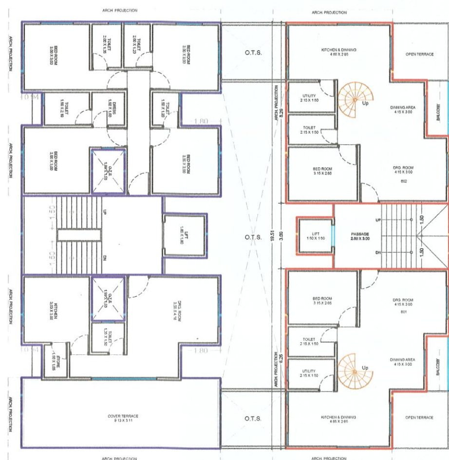
PROP. EXTN. 6TH FLOOR PLAN BUILT UP AREA : 123.78 SQ.MT F.S.I. AREA : 104.90 SQ.MT.
