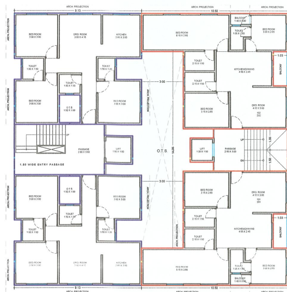
PROP. EXTN. 1ST & 2TH FLOOR PLAN BUILT UP AREA : 154.09 SQ.MT F.S.I. AREA : 135.20 SQ.MT.
