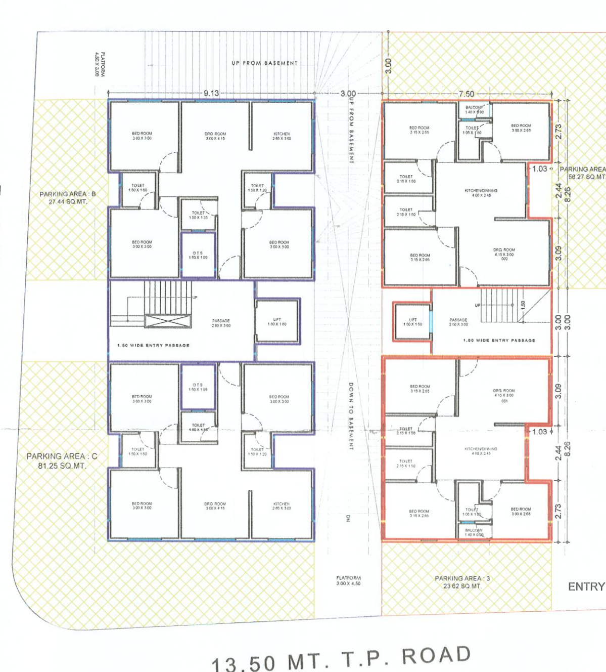
GROUND FLOOR PLAN BUILT UP AREA : 137.72 SQ.MT. F.S.I. AREA : 116.84 SQ.MT. PARKING AREA : 113.62 SQ.MT.
